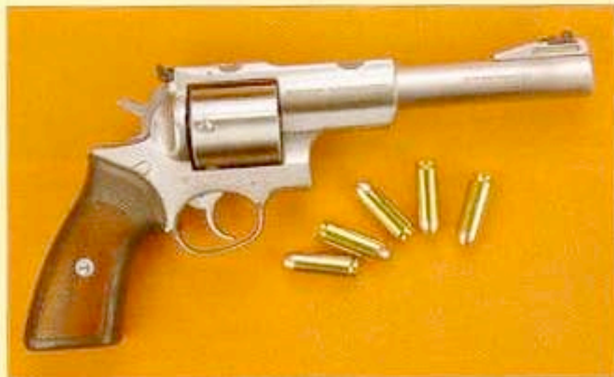
The full-size .50 AE conversion features a five-shot unfluted cylinder and a 6½ barrel. Although we fired it using the excellent fully adjustable sights, the gun features Ruger's integral scope bases.
