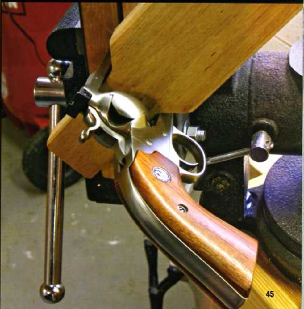
The industrial-strength barrel vise with its contoured brass inserts is usually found only in a working shop. It is capable of exerting tremendous pressure and can damage barrels if used injudiciously. A wooden action wrench (below) works very well for single-action revolvers and won't mar the finish. One a couple of feet long provides ample leverage to overpower all but the tightest barrels — provided the barrel doesn't spin in the vise.
