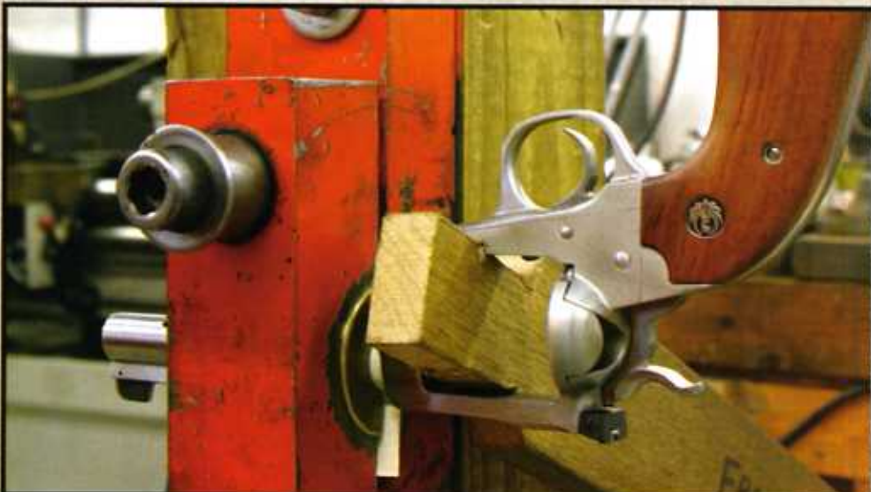
The industrial-strength barrel vise with its contoured brass inserts is usually found only in a working shop. It is capable of exerting tremendous pressure and can damage barrels if used injudiciously. A wooden action wrench (below) works very well for single-action revolvers and won't mar the finish. One a couple of feet long provides ample leverage to overpower all but the tightest barrels — provided the barrel doesn't spin in the vise.
