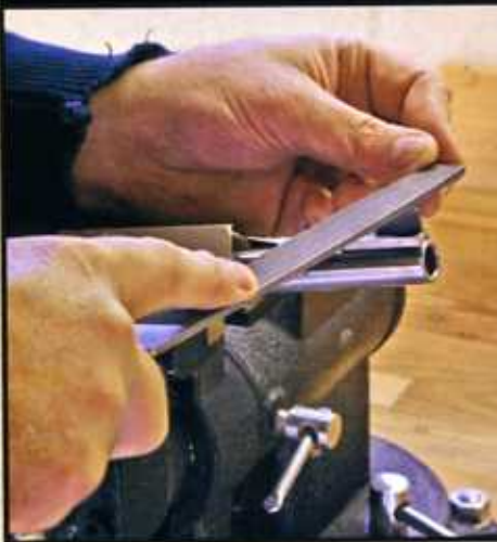
The things backyard barrel vises are made of (above). Materials should be readily available just about everywhere. Filling the blade to height and shape (below, left) is not as easy as it looks if you haven't done a few thousand of them. Go slow and check your work often since it is much easier to remove material and replace it. This is what it looks like (below, right) once all the bits and pieces are assembled with the barrel in place.
